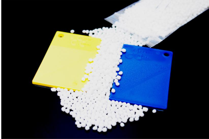
Another important factor is dispersion. Studies have shown that inconsistent dispersion of colorant can negatively impact performance characteristics of the final part. The biggest single threat is that improper dispersion can interfere with molecular bonds, “resulting in pigment agglomerates acting as defects in the polymer matrix and impairing the mechanical properties of the finished product.”<sup>1</sup> Thus, consistent dispersion is crucial when pigmenting PCR.
